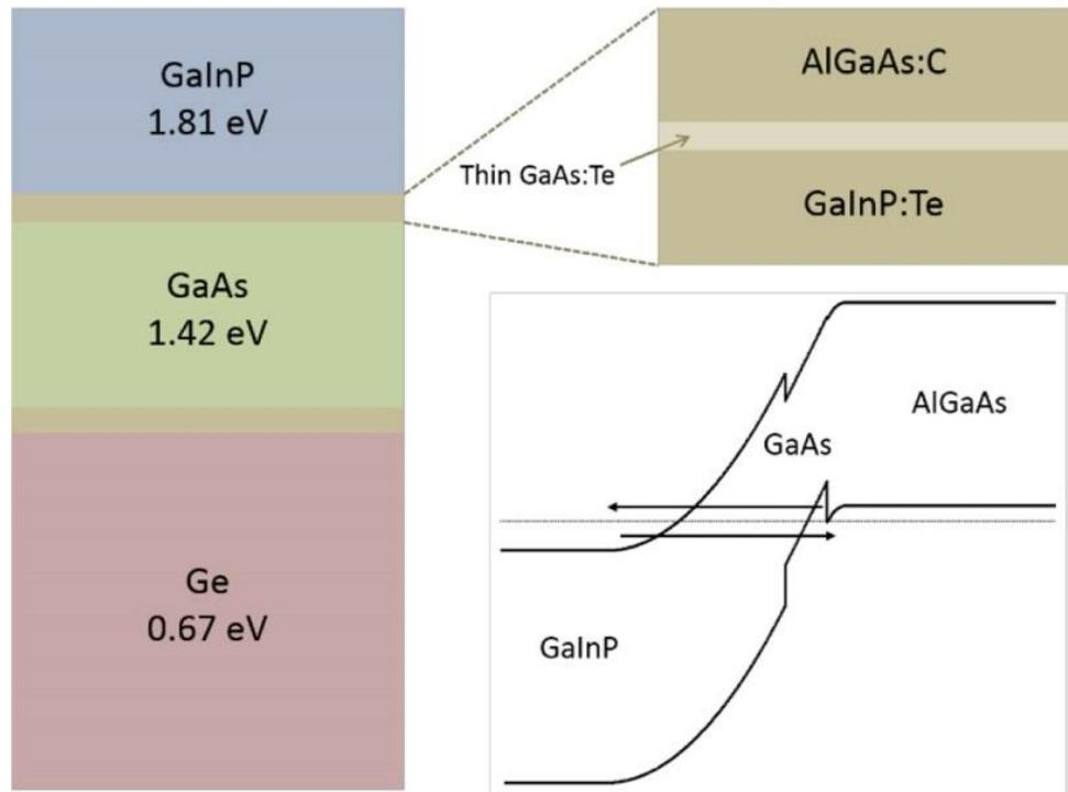
**Figure 1.** Location of the new tunnel junction (TJ) structure in a multijunction (MJ) solar cell. Also shown is the band diagram for a TJ with a 30Å gallium arsenide (GaAs) layer. GalnP: Gallium indium phosphide. Ge: Germanium. AlGaAs:C: Carbon-doped aluminum gallium arsenide. GaAs:Te: Tellurium-doped GaAs. GalnP:Te: Tellurium-doped GalnP.
