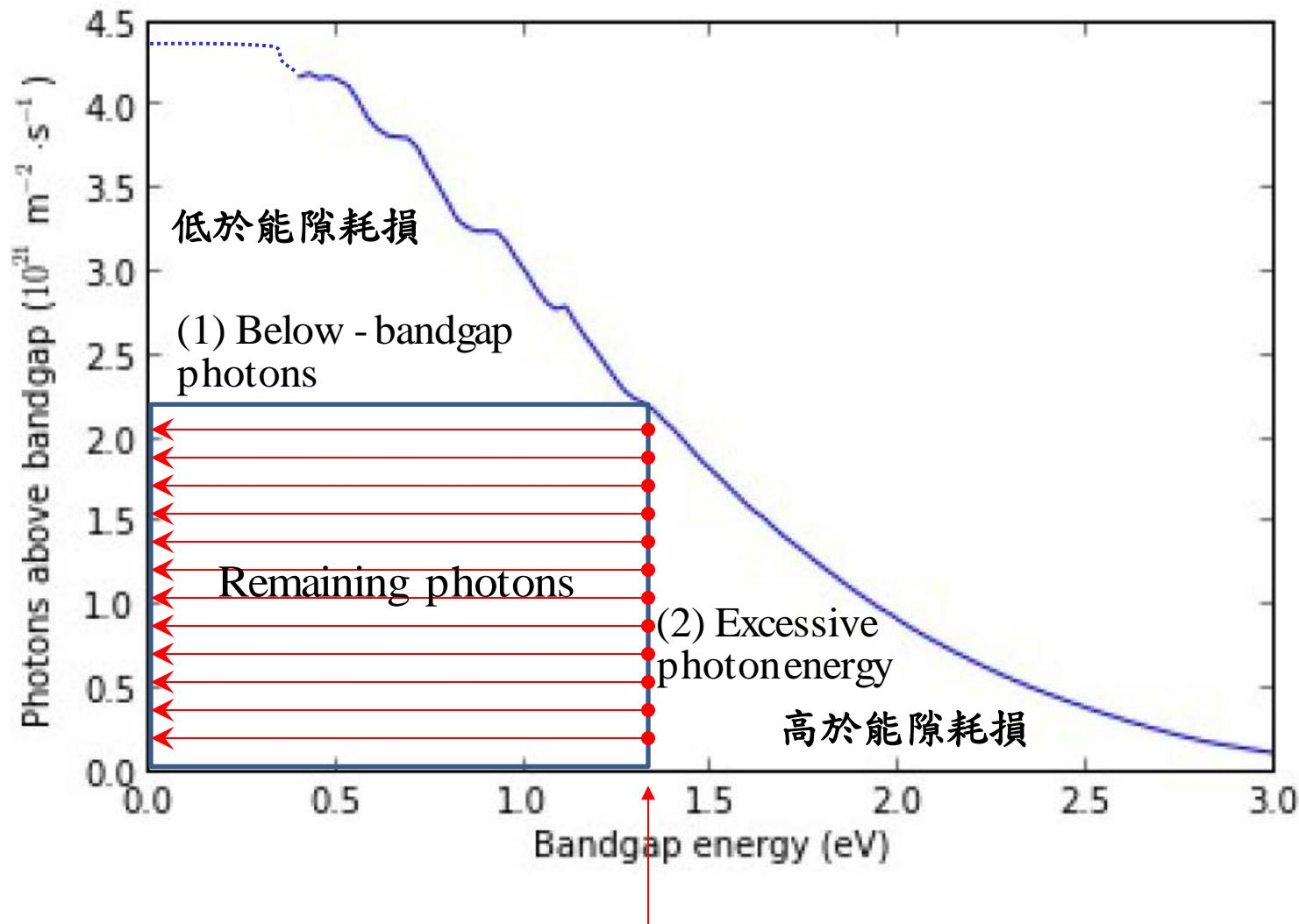
Assumes a single p-n junction diode solar cell with bandgap equaling 1.34 eV.
